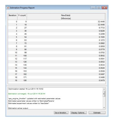
The estimated parameters are saved in the Parameter Estimation tool, in the **Results** section of the **Data Browser** pane, as EstimatedParams. Right-click EstimatedParams, and select **Open...** to view the results.
