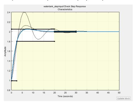
The plot displays the last five iterations. The final response using the optimized variable parameter appears as the thick blue line. The optimized response lies in the white region bounded by the design requirement line segments and thus meets the requirements.
