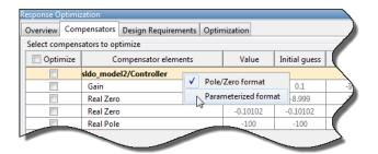
The controller parameters now display as Simulink block mask parameters, P, I, and D. For more information, see "Design Linear Controllers for Simulink Models". To learn more about mask parameters, see "Mask Parameters" (Simulink).
