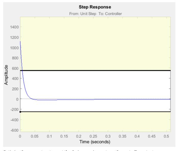
**3** Optimize the parameters to meet the design requirements on the controller output:
