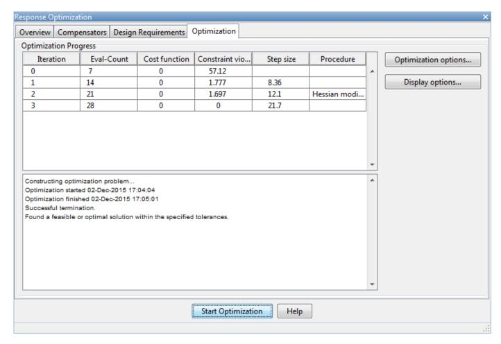
The status message, Successful termination, indicates that the optimization method found a solution that meets the design requirements. For more information about the outputs displayed in the **Optimization progress** table, see "Iterative Display" (Optimization Toolbox).
