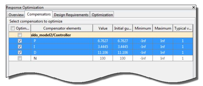
b In the **Optimization** tab, click **Start Optimization**. At every optimization iteration, the optimization method reduces the distance between the current response and the upper and lower bounds on the signal. After the optimization completes, the **Optimization** tab displays the optimization iterations and status.
