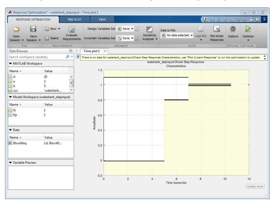
The region bounded by black line segments in **Time plot 1** shows the step response requirements that you specified in the Check Step Response Characteristics block.
