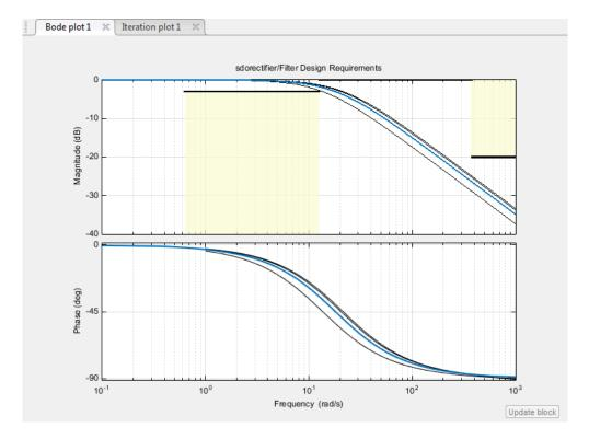
The plot displays the output of the last five iterations. The final response using the optimized parameter values appears as the thick blue line.
