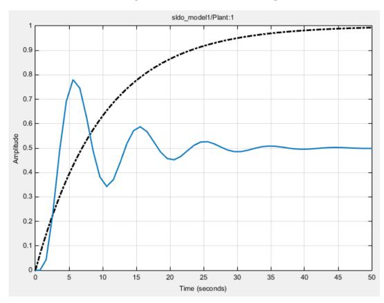
The plot shows that the model response does not track the reference signal.
