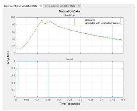
**a** Examine the experiment plot to see how well the simulated output matches the output data.
