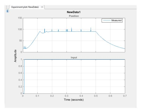
The time plot shows the output data in response to a step input, as described in "About the Sample Data" on page 2-3. The plot shows a rapid decrease in the response after t=0.5 s because the system is shut down. To focus parameter estimation on the time period when the system is active, select the data samples between t=0 s and t=0.5 s, as in "Extract Data for Estimation" on page 2-6.
