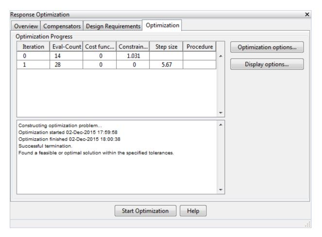
The status message, Successful termination, indicates that the optimization method found a solution that meets the design requirements.
