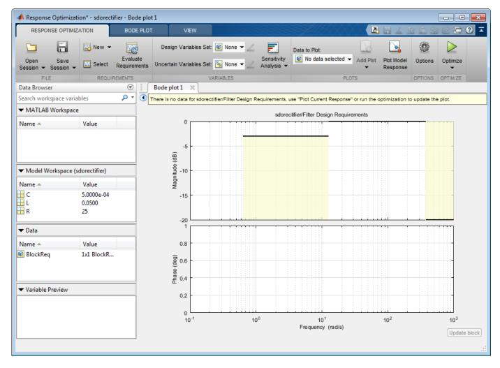
The **Bode plot 1** tab shows the gain and bandwidth requirements specified in the Filter Design Requirements block in the model. To see their values, double-click the block to open the Block Parameters dialog box, and select the **Bounds** tab.
