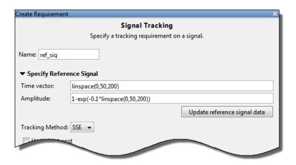
Leave the **Tracking Method** as SSE which means, at each optimization iteration, the solver attempts to reduce the sum of squared errors between the simulated output and reference signal.
