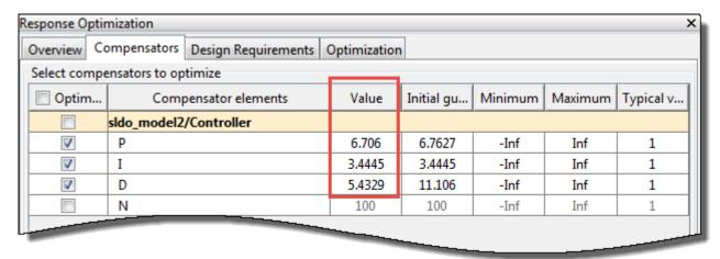
6 Write the optimized controller parameter values to the Controller block in the Simulink model.
