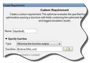
A new requirement variable MaxMinRL is created, and appears in the **Data** area in the Response Optimization tool. The **Iteration plot 1** tab shows the value of MaxMinRL at each iteration during the optimization.
