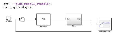
The model includes a Step Response block which is a Check Step Response Characteristics block from the Simulink Design Optimization **Model Verification** library and has default step response bounds.
