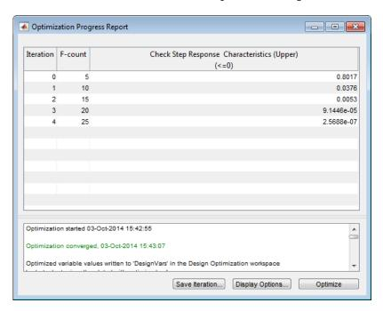
The message Optimization converged in the Optimization Progress Report indicates that the optimization solver found a solution that meets the design requirements within the tolerances and parameter bounds. For more information about the outputs displayed in the optimization, see "Iterative Display" (Optimization Toolbox).
