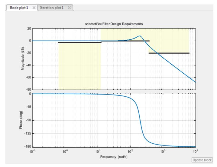
The **Bode plot 1** window in the Response Optimization tool shows that the model output goes out of the region bounded by the design requirement line segments.
